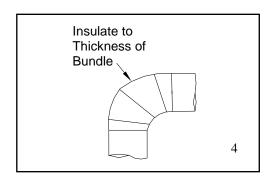
5. Cover with a weatherproof jacket. A Dekoron-Unitherm Seal Patch Kit (p/n 1540-10000 or 1540-20000) has the items necessary to correctly insulate and jacket the bundle.
