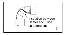
4. Replace the thermal insulation over the heater until the overall insulation is the same thickness as originally found on the bundle.
