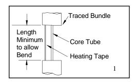
2. Make the bend required in the tubing using a suitable mandrel. Again, take care not to damage the heater or tape. A standard tubing bender can be used for this task but care must be taken to insure the heater is not stretched or cut during the bending process.
