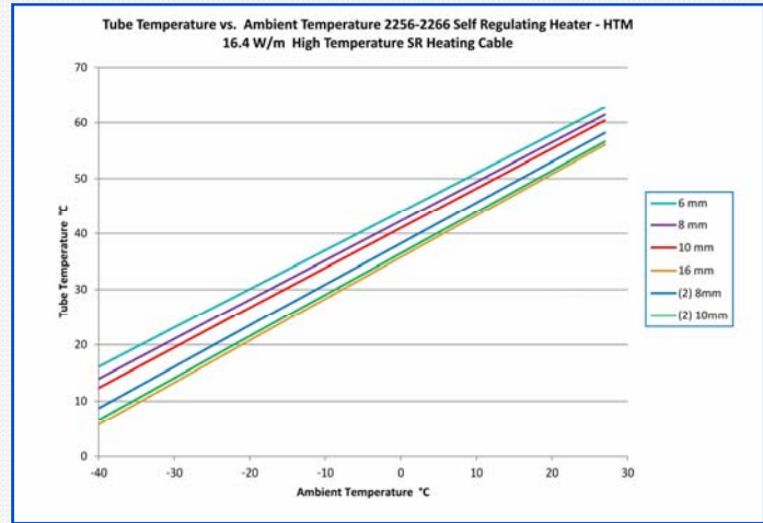
Tube Temperature vs Ambient for standard bundles with 16.4 w/m HTSR
